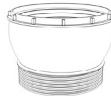
4 Junction upper section with adjustable socket
