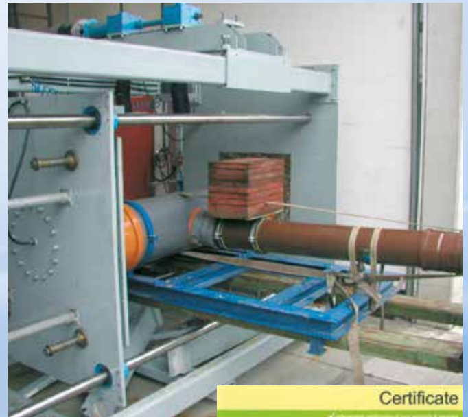
Test set-up for shear loading test
