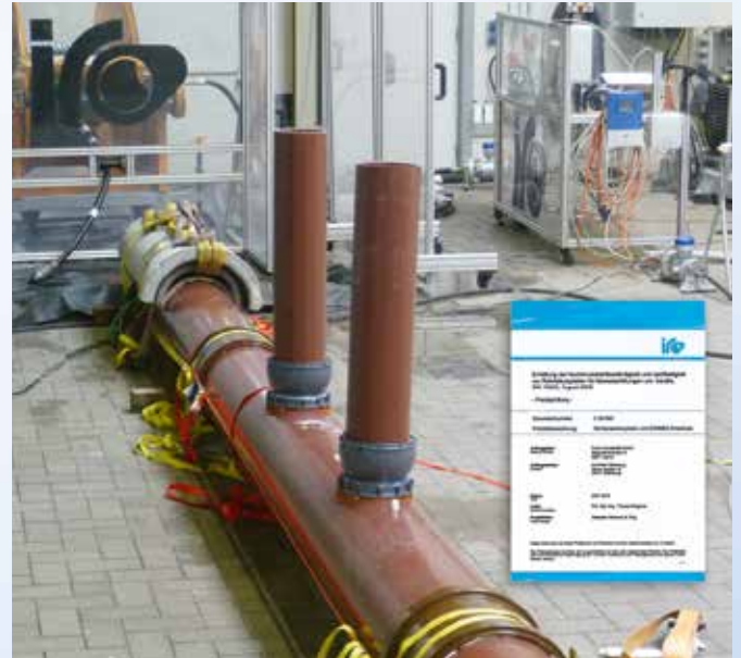
Jetting test iro 19523
