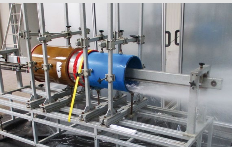
High-pressure water jet test in accordance with DIN 19523 at iro GmbH Oldenburg
