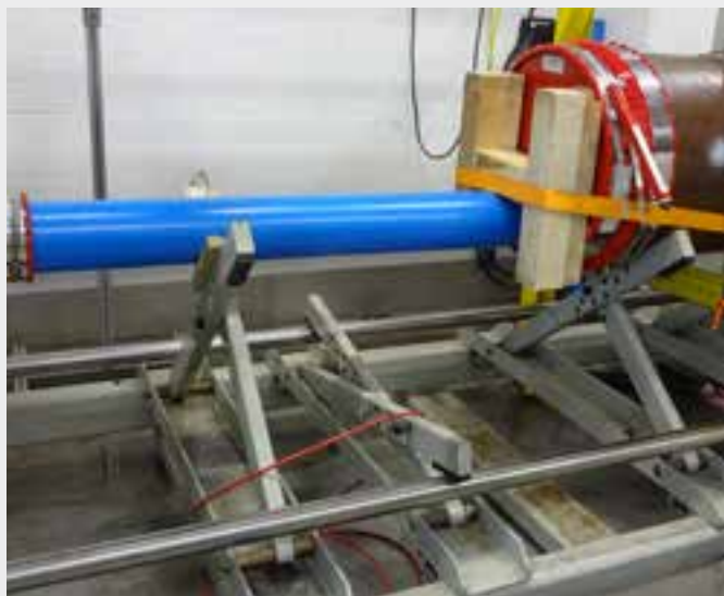
Internal leak test according to DIN 4060 in Funke's own test rig.
